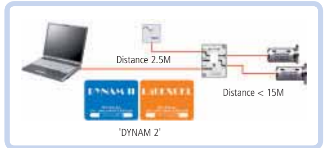
Connection to a PC/laptop through a T/C (Transceiver/Converter)
