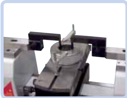
Checking of ring gauges
