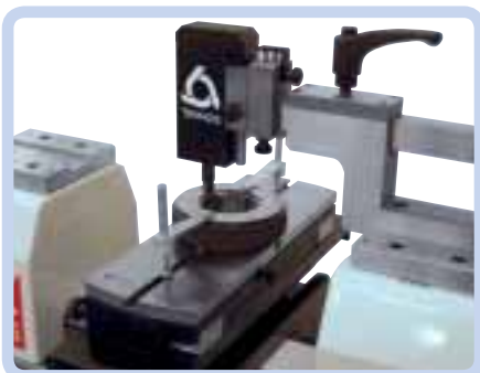
Checking of screw ring gauges
