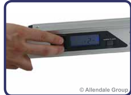
3. Press the calibration button(s), to start the second angle measurement. Once this reading taken the level will calculate true level. Please note: The level will not calibrate if movement or vibration is detected during the calibration procedure.
