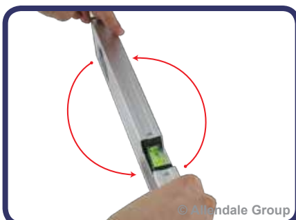
2. When the level has stored the first measurement the display show "-2-" or "-H-". Rotate the level 180 degrees on the flat surface.
