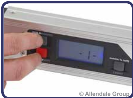
1. Press and hold the calibration button(s) Release when the display shows "-1-" or "-H-". Whilst the display is flashing, an angle measurement is being processed. Do not move the level. Please note: On the ME-AN-LEV-600 model, press and hold the ON/OFF. This will enter calibration on the next power up. Press C button to start calibration.
